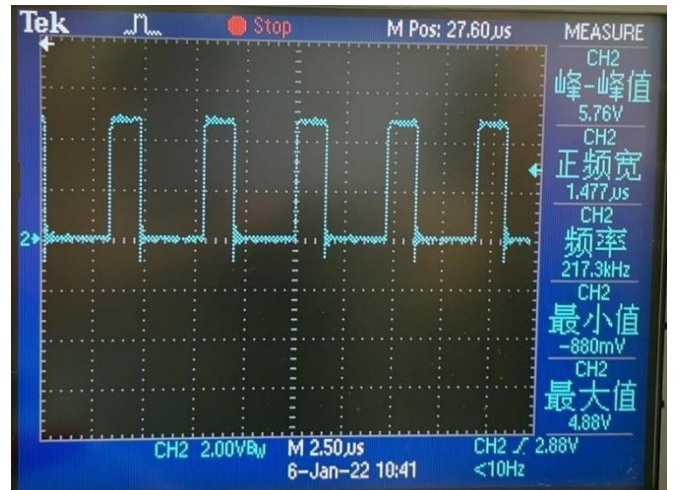
MOS switch waveform
